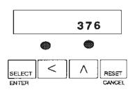
After one of these options is displayed for a second, the value for this option is automatically displayed. Once the option value is displayed, pressing the < key will move one digit to the left and the  $\Lambda$  key will increment the value by one. Then the SELECT key must be pressed
